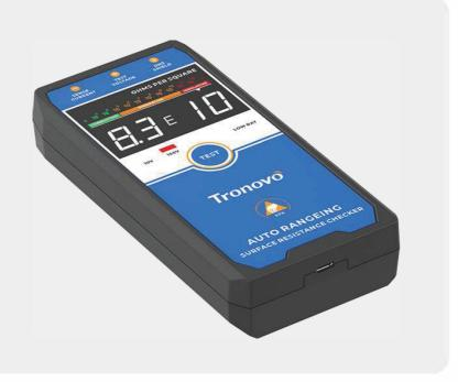
The MR43 is an affordable and reliable surface resistance tester for checking surface resistance and ground resistance. Pressing the test button automatically generates a test voltage of 10V or 100V, and the instrument can be used for performance evaluation tests on different work surfaces, floors, chairs, carts, clothing, and packaging materials. Measurements can be made using the built-in measuring electrode on the bottom of the instrument, or in combination with other probes.
